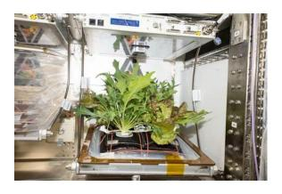
In the absence of gravity, plants use other environmental factors, such as light, to orient and guide growth. A bank of light emitting diodes (LEDs) above the plants produces a spectrum of light suited for the plants' growth. Since plants reflect a lot of green light and use more red and blue wavelengths, the Veggie chamber typically glows magenta pink.
